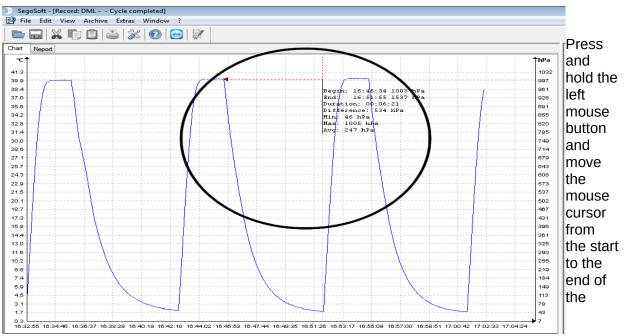
measured curve section and release it. The measured numerical values for time and temperature or time and pressure appear. The resulting document can be saved as a file with "File/Create PDF".
